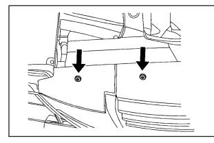
2. Remove the two screws from the top of the front fascia and grille. They are inboard of the headlamp assembly.
